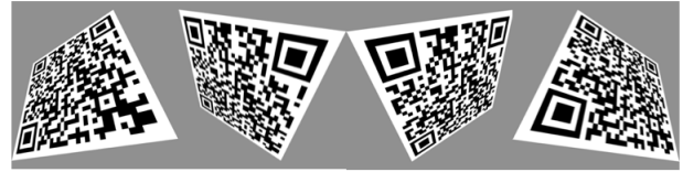
(a) Each assignment of \pm 38^\circ inclination applied along x - and y -axes. QR code readability is highly asymmetric.
